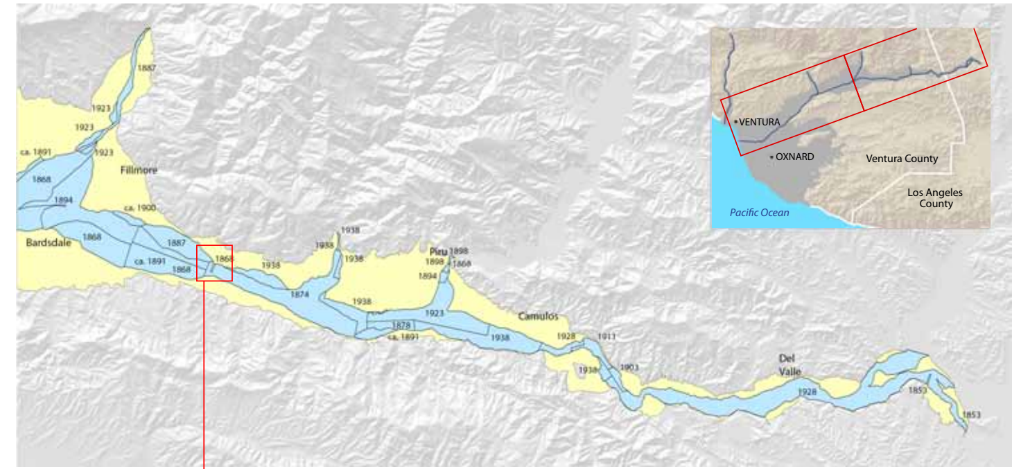
Fig. 3.14. Location of the Santa Clara River corridor by earliest available source, 1853-1938. We mapped the historical position of the outer bank, using the earliest data found for each stretch of the river. We found that while large flood events caused locally significant adjustments in outer bank position and total river corridor width, these changes were relatively small at a regional scale. Pull-out quotes provide examples of the types of sources used to map the historical river corridor.
